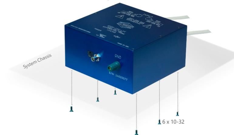
DP30 series probes can be mounted directly on a base plate or enclosure walls with 6 x 10-32 screws.
