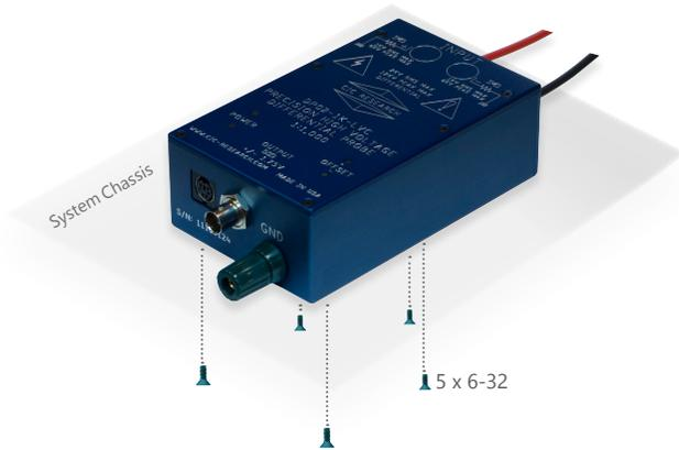
DP02 series probes can be mounted directly on a base plate or enclosure walls with 5 x 6-32 screws. Optional mounting flange models are available, shown below. These can be mounted with 4 x 10-32 (or M5) screws.
